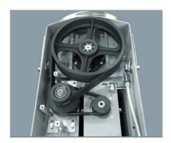
Premium drive system provides more torque on the machine
