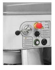
3M - Panel with 3 speed mechanical gearbox and mechanical timer
