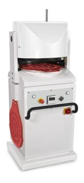
Hammonia Bun Divider and Rounder is available in fully automatic and semi-automatic. An up-to-date bun divider and rounder has to be:
